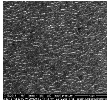
Fig. 4 Morphology of Be target after interaction with plasma air plasma
