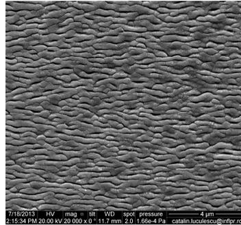
Fig. 2 Morphology of W target after interaction with plasma air plasma
