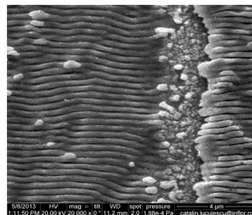
Fig. 5 W target surface morphology after laser indirect irradiation in D2 atmosphere.
