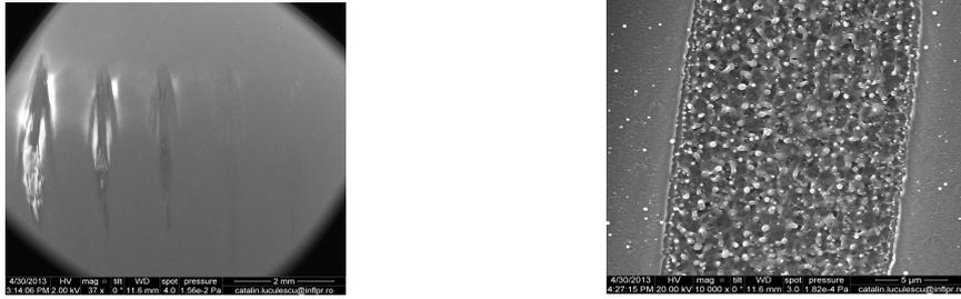
Fig. 6 Carbon target morphology after laser indirect irradiation in D2 atmosphere.
