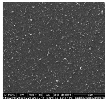
Fig. 3 Morphology of C target after interaction with plasma air plasma
