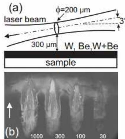
FIG. 1. (a) The laser beam is focused in a spot with diameter  $\phi$  near the samples coated with Be, W, and C (b) SEM images of craters on the Be surface produced in air after firing 1000, 300, 100 and 30 laser pulses, respectively. The arrow indicates the laser beam direction.
