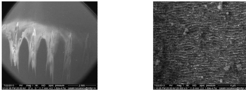
Fig.7 Be target morphology after interaction with plasma produced by laser in D2 atmosphere.
